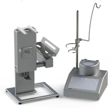
Impromediform GmbH is proud to present the very first intelligent peristaltic pump managing a high precision volumetric delivery solution with the live support of an integrated high-resolution scale.
